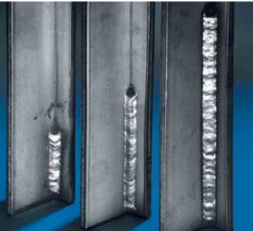
Deposition rate from Shield-Bright cored wires in positional welding outperforms MMA electrodes and solid wires, shown here for one minute welding in the PF (3F) position.
