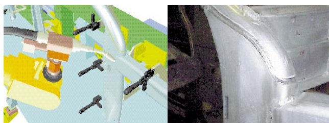
Figure 6. Detailed study of a 3D MIG joint and the corresponding result after welding.
