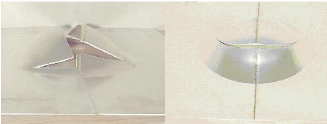
Figure 11. Cracking behaviour of welded aluminium blanks.
