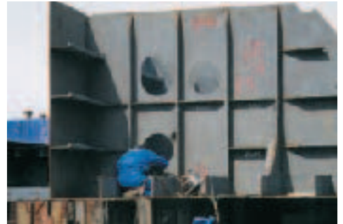
Figure 10. Outdoor FCAW with PZ6116S.
