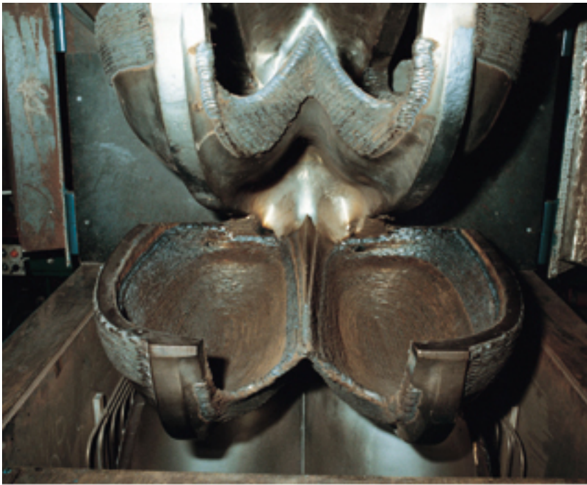
Figure 6. Pelton wheel buckets after rebuilding with PZ6166
