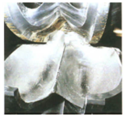
Figure 3. Pelton wheel buckets with characteristic wear pattern.
