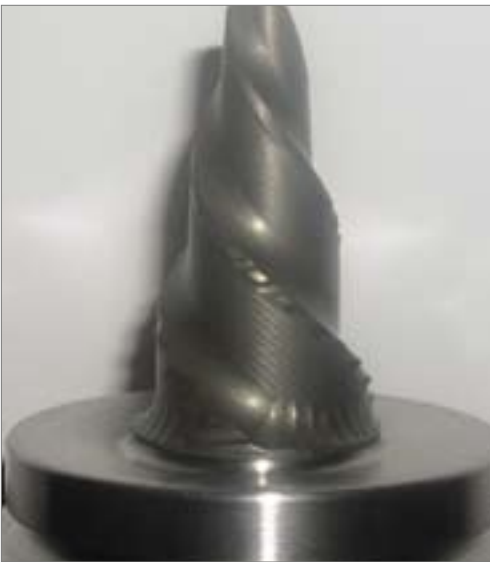
Figure 3. The tool probe and shoulder.
