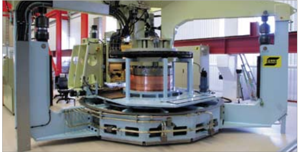
Figure 4. The welding machine at the Canister Laboratory.
