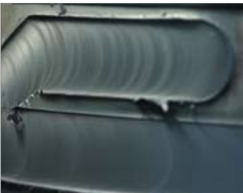
Figure 6. Parking of the tool during the bottom weld of a full size canister.
