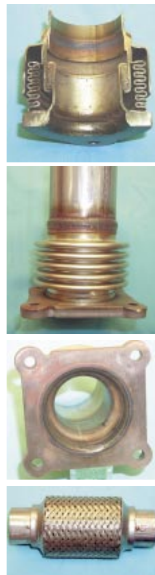
Figure 1. Automotive exhaust components welded with 1.2 mm Arcaloy 18CrCb showing joint complexity and
