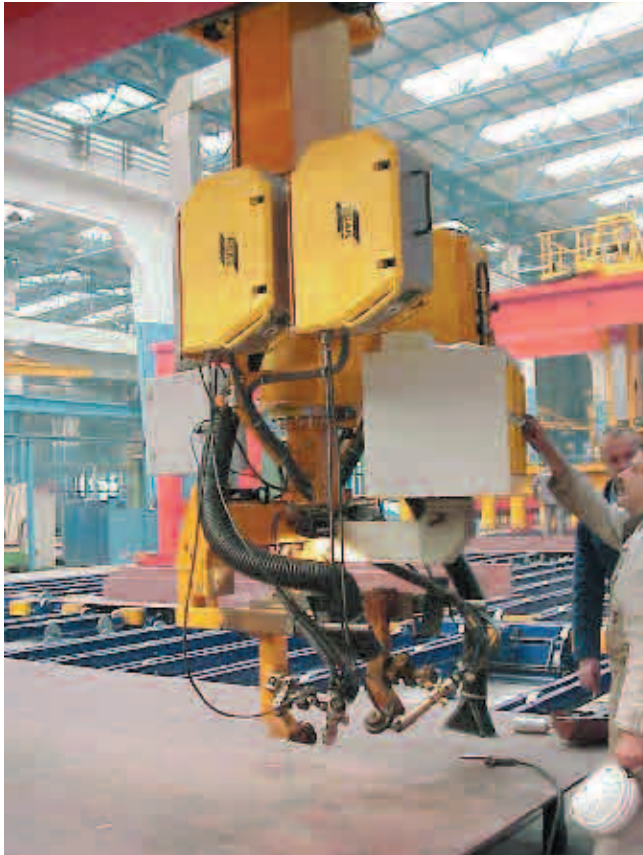
Figure 4: ESAB's tandem welding system at the Kværner Shipyard in Rostock
